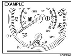
When you press the engine switch to change the ignition mode to "ON", this gauge gives an approximate indication of the amount of fuel in the fuel tank. "F" stands for full and "E" stands for empty.
